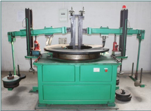
转盘式脚轮测试机 Turnplate Caster Lifetime Tester
