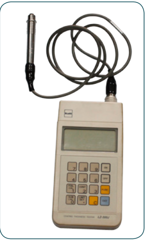
涂镀层测厚仪 Coating Thickness Tester
