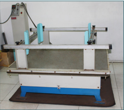
模拟运输振动试验机 Packing Vibration Stimulate Equipment
